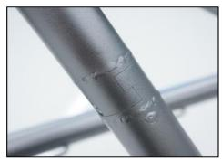
Precision-machined tube joints for rear two supports. TIG welded 360 degrees + plug welded. A seriously strong joint that is far superior to through-bolted slip-fit tubes.
