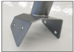
Bolts to the Ford-engineered corner gussets with heavy 1/8" thick steel plate. Don't risk the strength of your car to flimsy aftermarket gussets.
