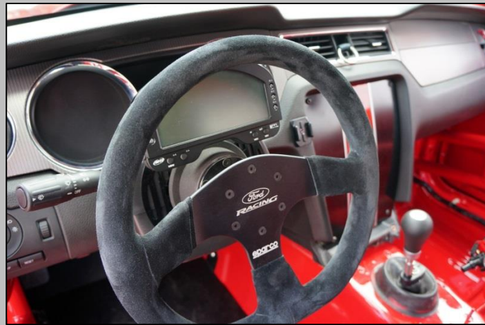
Sparco quick release steering wheel & optional AIM system. Gauge delete panels, short-throw shifter.
