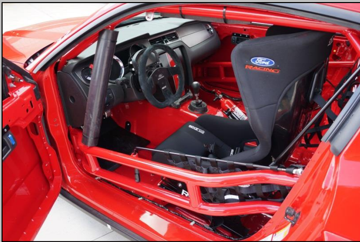
Fully painted interior with sound deadening removed.
