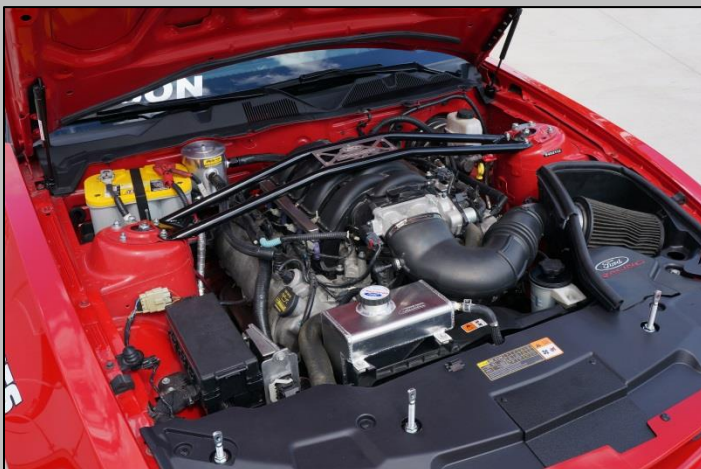
Ford Racing Cold Air Intake + Tune, Strut tower brace. Hood Struts, Watson Hood Pins welded to rad support.
