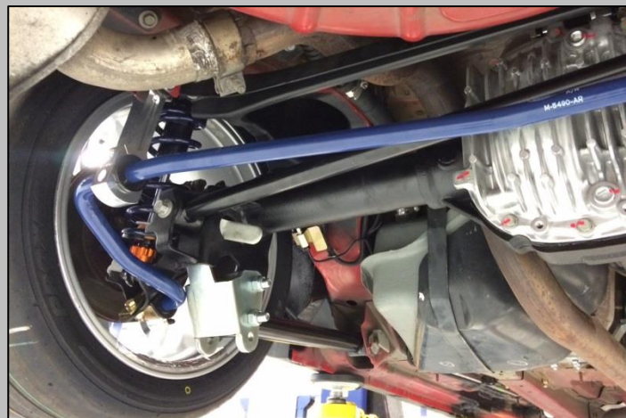
FRPP suspension components + diff cover, HVT coil-over suspension.
