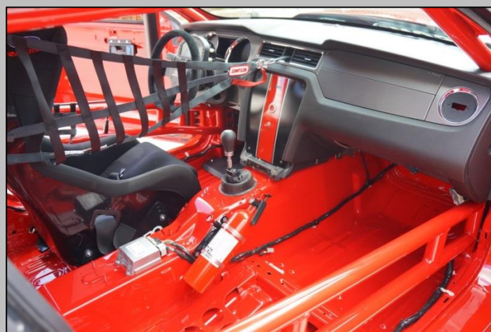
Clean and orderly. Fire bottle within reach. Optional Driver's interior net and sound deadening removal.
