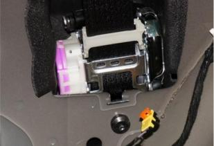
12) Remove the (3) 13mm bolts on either side of the car. Remove any seam sealer around the corner brace-to-floor area that may interfere with a roll bar.
