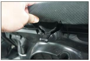
3) Remove rear seat back cushion by removing three 15mm nuts/bolts total- one left, right, and center, bolting hinge brackets to floor, then pulling the release straps at the top.
