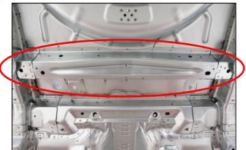
21) Use the spot welds for the beam under the car as a reference for centering the pads.
