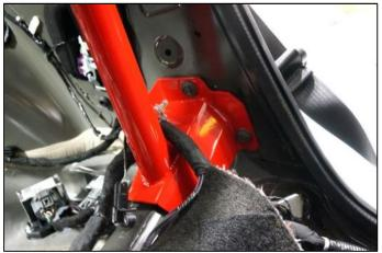
16) With the bar in place, start the (6) M8 x 30mm bolts provided, but do not tighten. As noted in step #13, you may need to clearance the roll bar to allow the bolts to seat properly. NOTE that the ground wire bolt locations may interfere with the roll bar as well, and may need clearancing (below). These issues have been addressed in later versions of the roll bar.
