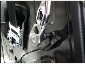
11) It may assist in freeing the harnesses to disconnect the seat belt crash tensioners on both sides. Use a small pick tool to carefully lift up on the orange connector lock, then lift up on the connector body. **NOTE:** It may be helpful to remove the same connectors from the seat belt retractors as well (right picture, below).
