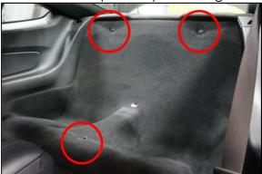
6) **GT350R:** "Un-stick" OEM Velcro from plastic trim panels, used to hold edges of Seat Delete Panel in place. Leave Velcro stuck to the carpet for later re-use.
