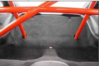
42) Start the (8) M10 flange bolts in the feet of the diagonal bars. Fully tighten these as well as the machined joint bolts once all have been started.
