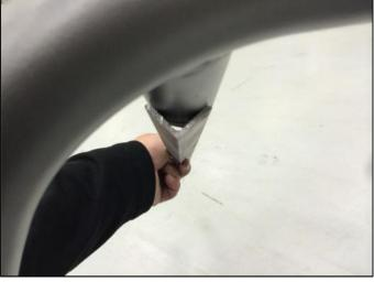
41) Once your holes are cut, insert the rear two diagonal bars through the trunk, through the seat delete panel, and install to the roll bar's main hoop.
