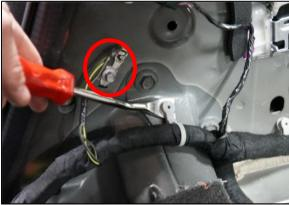
10) Remove the impact sensors by removing the 8mm bolts. Retain for re-installation.
