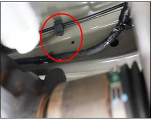
24) With the brake lines dislodged, drill the 6 holes per side from inside the car. Start with a 1/8" pilot for all holes. The two center holes should then be drilled with a 1/4" bit, and the four outer holes with a 1/2" bit. Vacuum shavings from the car.
