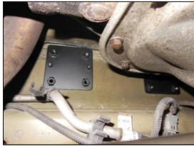
18) Install Watson 4-point Roll Bar into place using provided M10 bolts. With all 8 forward Roll Bar bolts **only started** (not tightened) tighten all factory gusset bolts. Use of threadlocker is advised on both gusset bolts and Roll Bar bolts. Leaving the Roll Bar's bolts loose may aid in the installation of the rear diagonal bars, which are installed later. \*\*See step #25 regarding torque specs.
