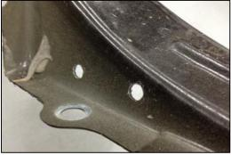
10) Return gussets to car and align with original bolt holes. Fasten with some of the bolts removed previously if needed.
