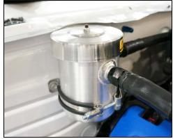
2) **PCV Lines**. Remove the factory PCV lines that connect the cam covers to the intake manifold and intake tube. Cap ports on manifold and intake tube with provided rubber caps and constant tension spring clamps.
