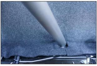
5) Install lower halves of carpet kit, starting with passenger side. Place panel all the way rearward in the car, and align forward push pin with hole identified in red circle, located at the front of the seat base 'riser'.
