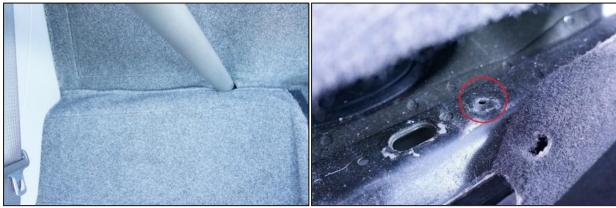
6) The carpet should have a hole for this push pin to pass through. Carefully feed pushpin through the carpet, and into the hole in the sheetmetal. Press or squeeze push pin into hole; do not force. If hole needs to be enlarged slightly, do so with the next size drill bit.
