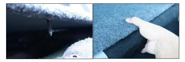
7) **Note:** Due to trim panel location variances from car to car, we've included some extra carpet material on the left/right outer edges of lower carpet panels. This extra material can be tucked under the side plastic trim panels for a clean appearance.
