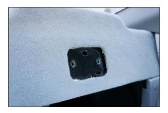
2) Place rear vertical carpet kit panel in car. Install the provided bolts through the pre-cut holes in the carpet kit, and notice how they align with one of the open holes where each latch was located.
