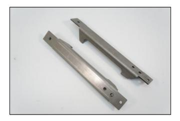
1) The Watson Racing 2015 Mustang Seat Mounts are now two separate "rails" allowing the flexibility to use any width race seat and some flexibility with its location. Note the rail spacing below:
