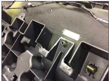
Watson Racing, LC 18703 Dix Toledo Rd Brownstown, MI 48193 855-928-7223 b) "Notch" the ends of the bumper support to accept tubular bumper. This will take some trial and error-insert the Watson tubular bumper (uninstalled) into the back of the fascia as a guide to direct your trimming.
