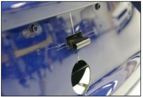
8) Install Ford Racing Tow Hook Loop (p/n M-17954-A), and you're ready to go racing!
