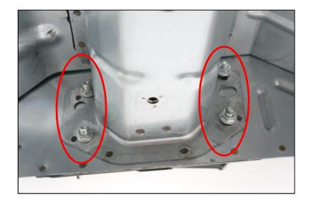
5) Install Watson Bumper using supplied M8x60mm flange bolts through the outer two holes on either end, and the supplied M8x35mm flange bolts on the inner two holes of either side. Capture these bolts with the supplied washers and M8 Nylock Nuts. Use the supplied M8x25mm bolts or the OEM bolts in the factory bumper bolt holes.
