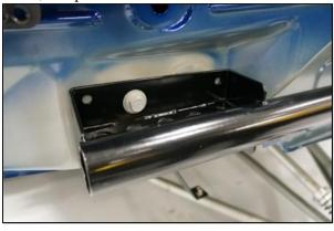
3) Mark the remaining 4 bolt holes on each side, to be drilled as noted in the next step. The factory bumper is only attached to the car with 2 bolts per side, which is NOT strong enough to sustain repeated abuse from parachute deployment.
