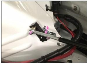
2) With fascia removed, remove factory bumper beam. Install supplied Watson Racing parachute bumper to the car using two of the original bumper bolts, one per side.
