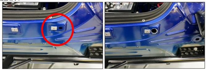
12) Drill matching hole in the plastic fascia retainer previously removed. Reinstall onto car, and route cable through.
