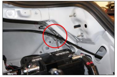
11) On the back of the car, remove center plastic fascia retainer. With a stepped drill bit, enlarge hole (circled) in sheet metal to 1".
