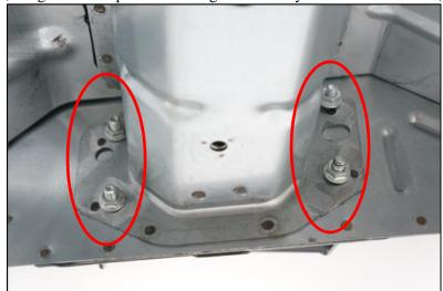
5) Install Chute Bumper using supplied M8x60mm flange bolts through the outer two holes on either end, and the supplied M8x35mm flange bolts on the inner two holes of either side. Capture these bolts with the supplied washers and M8 Nylock Nuts. Use the supplied M8 Socket Head bolts or the OEM bolts in the factory bumper bolt holes.
