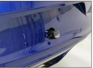
7) Drill 13mm hole for parachute release cable and the supplied cable grommet. This is optional- the instructions that follow show you a typical installation method for the chute release cable, but there are many options available to you. Epoxy grommet to fascia to lock it in place. Note that hole for cable is in-line with the cable holder on the Parachute Bracket. Second photo below is of the inside of the fascia, to aid in locating hole.
