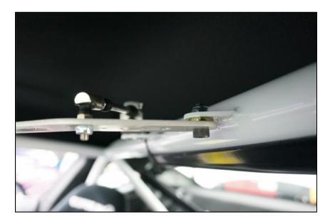
9) Route cable over roll cage tubes, secure to your liking using zip-ties. Dislodge C-Pillar trim panel, and route cable behind trim panel and down into trunk. Reinstall C-Pillar trim panel.
