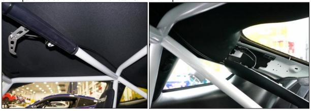
10) Route cable around passenger side of trunk. Use supplied P-clamp(s) wherever desired (circled). Note routing of cable through the existing hole in the sheet metal, below.
