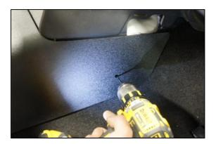
4) Drill all 4 holes with a 1/8" pilot drill bit. Enlarge to 1/2" with a step-drill bit or similar. Repeat all four holes.
