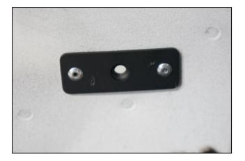
7) Install Console, secure to nut plates using provided socket head bolts. Apply a blue threadlocker to secure. DO NOT OVERTIGHTEN bolts!
