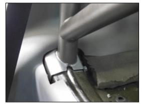
**NOTE:** As previously discussed, if you desire quick in/out access with trim panels installed, you will need to enlarge trim panel cuts to allow access to the Roll Bar's bolts.
