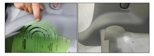
20) Clean up all cut lines and reinstall trim panels into car. Feed one panel at a time under the Roll Bar main hoop in the center, then work them forward between the Roll Bar and B-pillar. You will have to bend the lower portion of the trim panel to squeeze it between Bar and B-pillar. Use masking tape if desired to protect Roll Bar and trim panels from scratches. Panel should fit as it did originally; if not, check for clearance issues and trim further if needed.
