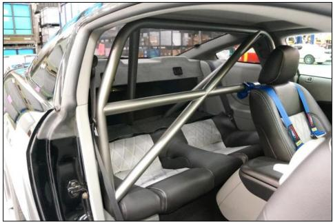
27) Seat lower cushion may be reinstalled if desired. Install shoulder harnesses through Roll Bar's belt retainer loops, and fasten/secure/buckle as per harness manufacturer's instructions. Enjoy your Watson Racing 4-point Roll Bar!
